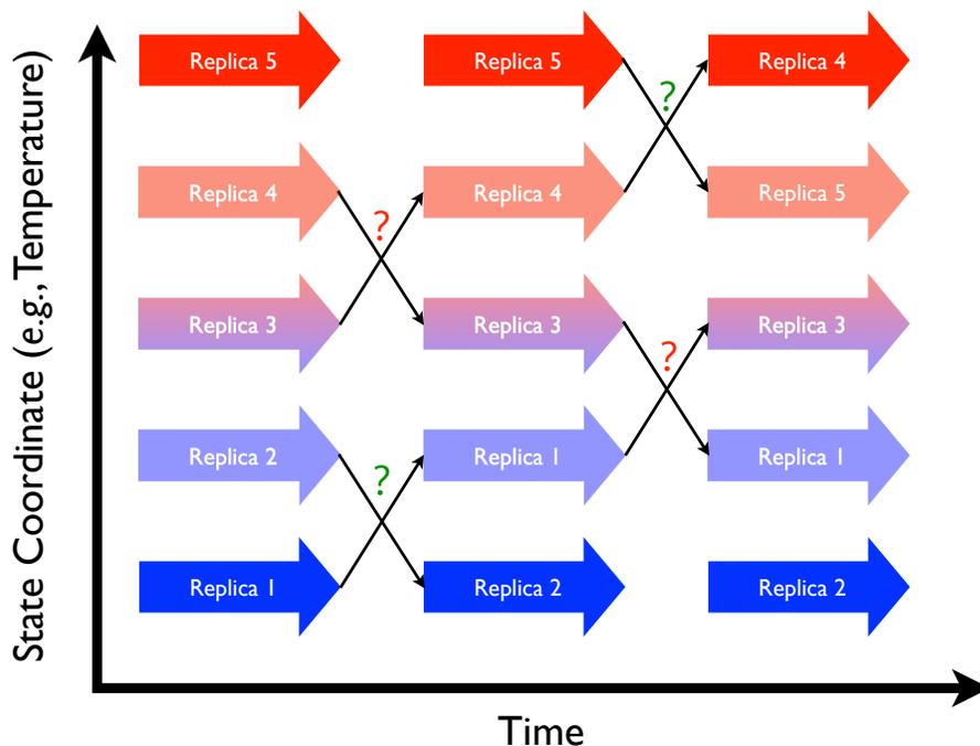
Figure 21.1.: *Replica exchange schematic showing 5 replicas combined in an expanded ensemble. Large arrows represent MD trajectories of sub-ensembles while the smaller arrows represent attempted swaps between replicas in state space. Question marks represent Monte Carlo exchange attempts (green for successful, red for failed).*
