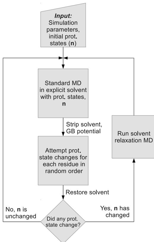
Figure 22.2.: Workflow for constant pH MD simulations in explicit solvent.
