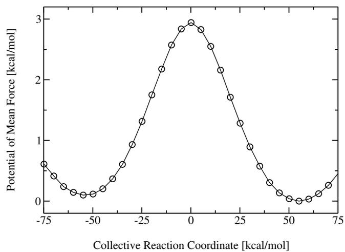
Figure 8.3.: *Potential of mean force for the intramolecular proton transfer in malonaldehyde as obtained from a series of umbrella sampling simulations along an energy gap RC. The distributions of the RC from all the windows are combined using the WHAM procedure.*
