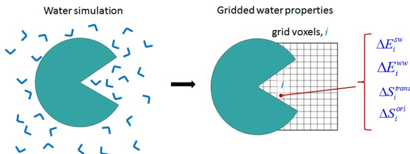
Figure 30.1.: Diagram, in 2D, of GIST's gridded water properties in a binding site.
