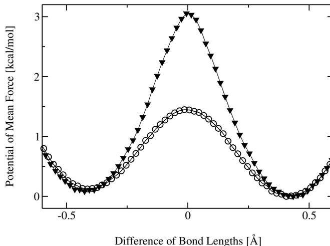
Figure 8.4.: PMFs as a function of the difference of bond lengths involving the proton with the donor and acceptor oxygens in malonaldehyde. The  $\blacktriangledown$  curve is from classical EVB, while the  $\odot$  curve is from EVB/PIMD.
